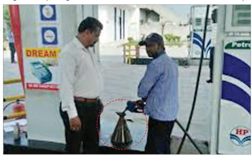
Fig. 2.1.19. Checked with the 5 litre measure
