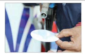
Fig. 2.1.15. Petrol evaporating from filter paper
