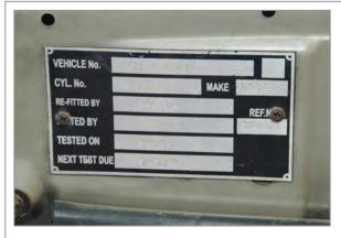
Fig. 3.2.1. CNG compliance plate
