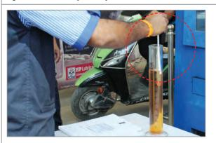
Fig. 2.1.20. Checking the density of a fuel
