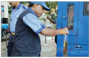
Fig. 2.1.19. Using calibrated hydrometer, thermometer
