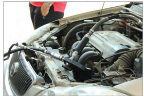
Fig. 3.2.3. Uncap the nozzle, before dispensing CNG
