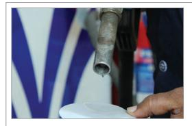
Fig. 2.1.14. Dispense a drop of petrol on the filter paper from the nozzle
