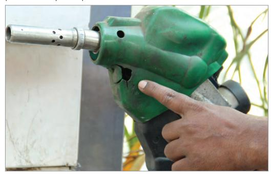
Fig. 3.2.2. Defective nozzle should be avoided
